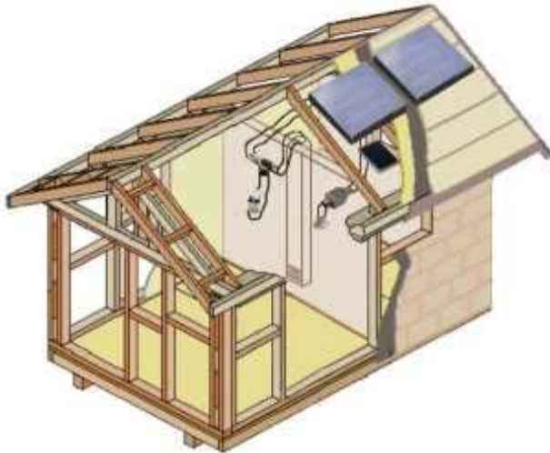
Example of a Solar Dual Climate Control System (Standard) on a House with a Ceiling Cavity
